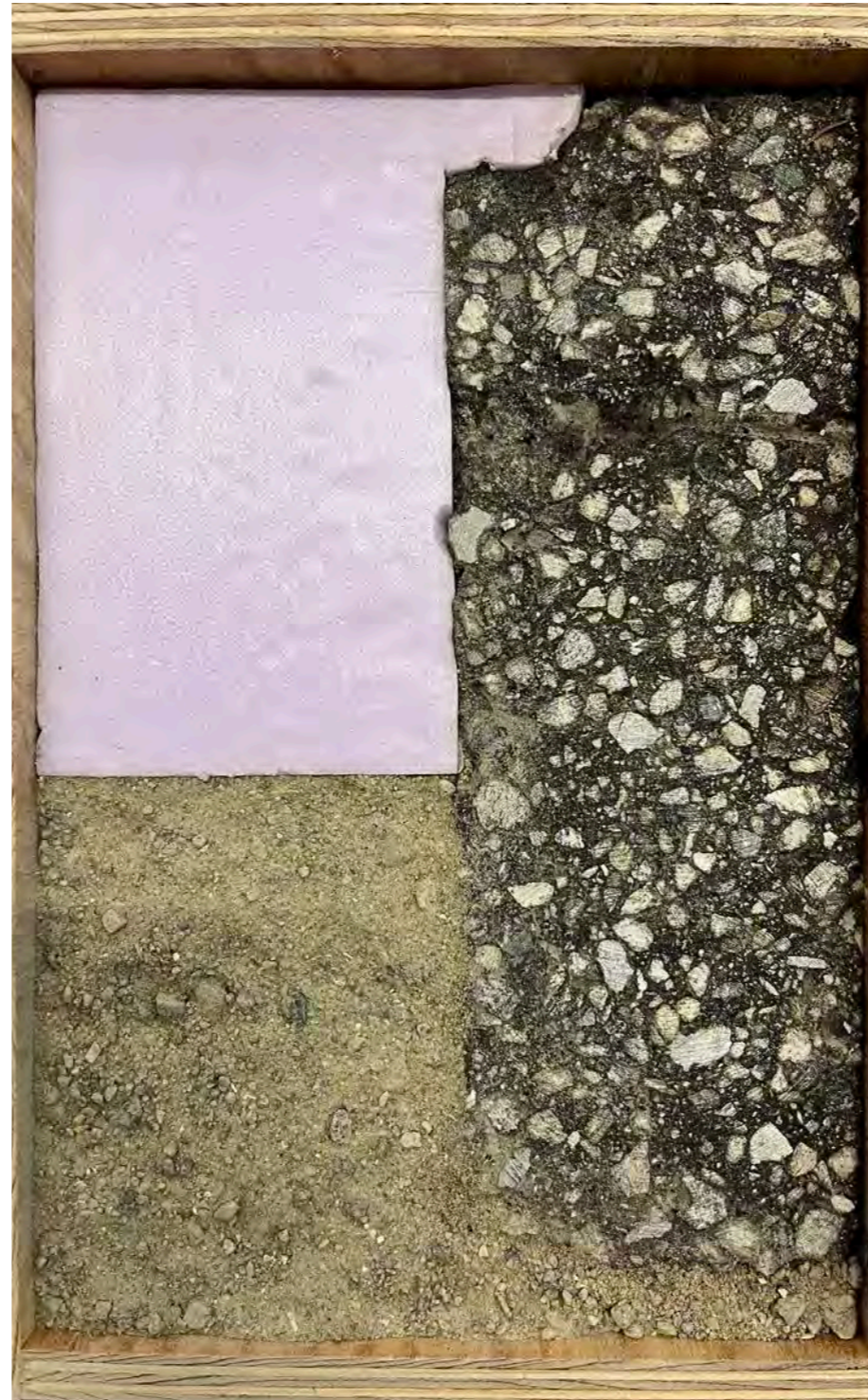
Asphalt, styrofoam and sand
